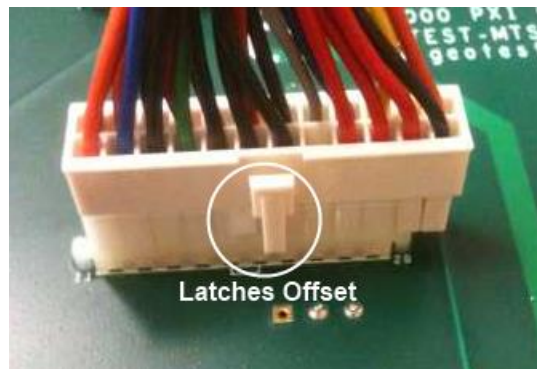
Figure 6: Latch is offset; RTV must be applied to secure the connector
