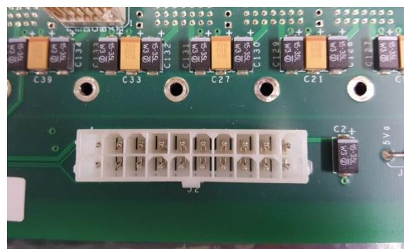
Figure 4: GX73xx Backplane Power Connector
