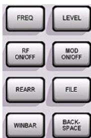
These keys provide direct access to the settings in the header of the instrument and can be used for fast changing the state of the modulation and the RF signal.
