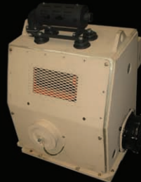
Multiple Launch Rocket System (MLRS) Auxiliary Power Unit
